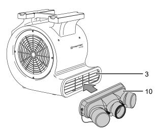
2. Move the attachment hooks (11) around until they are hooked into the air outlet grille (3).
