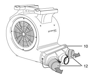
5. Connect suitable hoses (13) to the three-way hose distributor (10) and affix them using an appropriate hose clamp (14).
